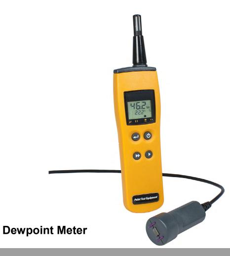
ISO 8502-4: Preparation of steel substrates before application of paints and related products. Tests for the assessment of surface cleanliness. Part 4: Guidance on the estimation of the probability of condensation prior to paint application.
